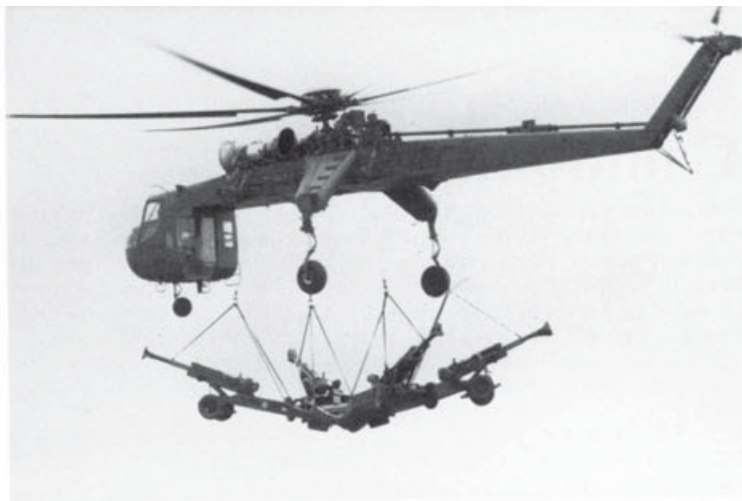
Various experiments were tried throughout the war in how to deliver supplies and equipment. This Skycrane lifts a whole battery of late model 105mm howitzers to see if such a technique is possible. (US Army)
