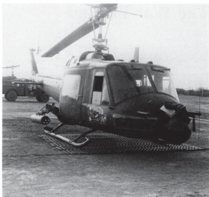
Newer weapons were added to gunships to increase their firepower. This UH-1B from the 120th AHC, the 'Razorback' Platoon, carries an XM-5 40mm grenade launcher mounted in its nose, and a set of 2.75 inch rocket launchers on the sides. (US Army)
