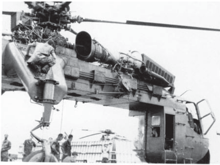
(Above) This CH-54 Skycrane shows off the maze of wiring and pipes which makes the big ship function. Constant maintenance was needed to keep these huge birds operational. (US Army)
