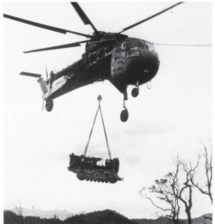
During the invasion of Cambodia Skycranes performed herculean cargo tasks as they flew in much needed equipment and supplies while removing captured material. This CH-54 lifts a bulldozer into an enemy base camp for use in demolishing enemy facilities. (US Army)
