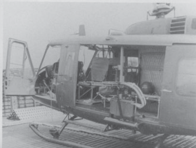
The standard M23 armament systems carried for the door gunners of both Huey slicks and gunships. The machine gun is an M-60D which was a modified version of the standard infantry gun. (US Army)
