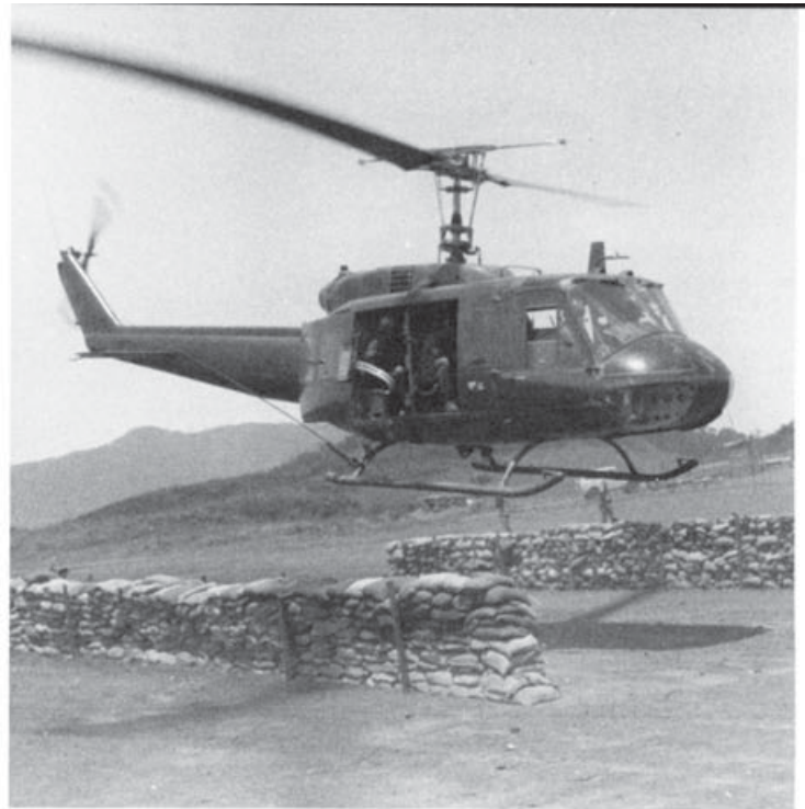
A UH-1D from the 1st Cav. lifts off a forward base for a mission into the An Alo Valley during PERSHING. Note the unusual antenna mount on the landing skid under the door gunner. (US Army)
