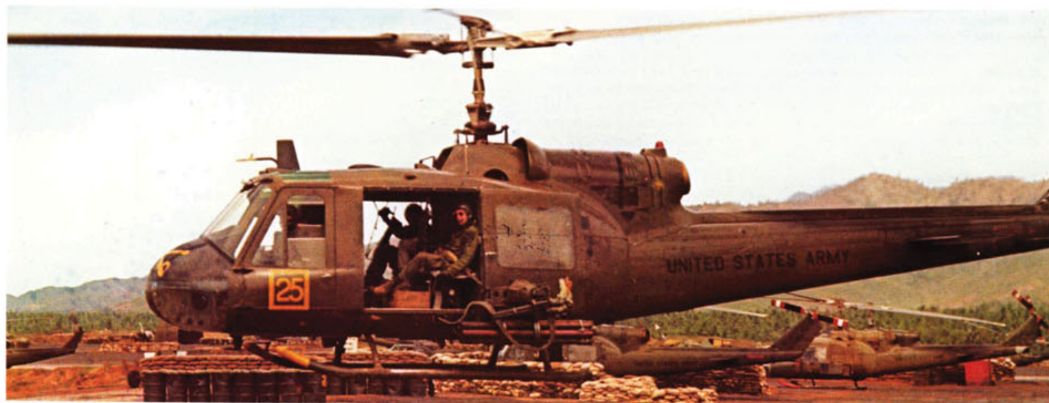
This UH-1C gunship takes off from LZ 'Two Bits' in the An Loa Valley. From 'B' Troop, 1st Squadron, 9th Cavalry, of the 1st Cavalry Division, it is fitted with the XM-158 rocket launcher and XM-50 mini-guns. (Mutza via Drendel)
