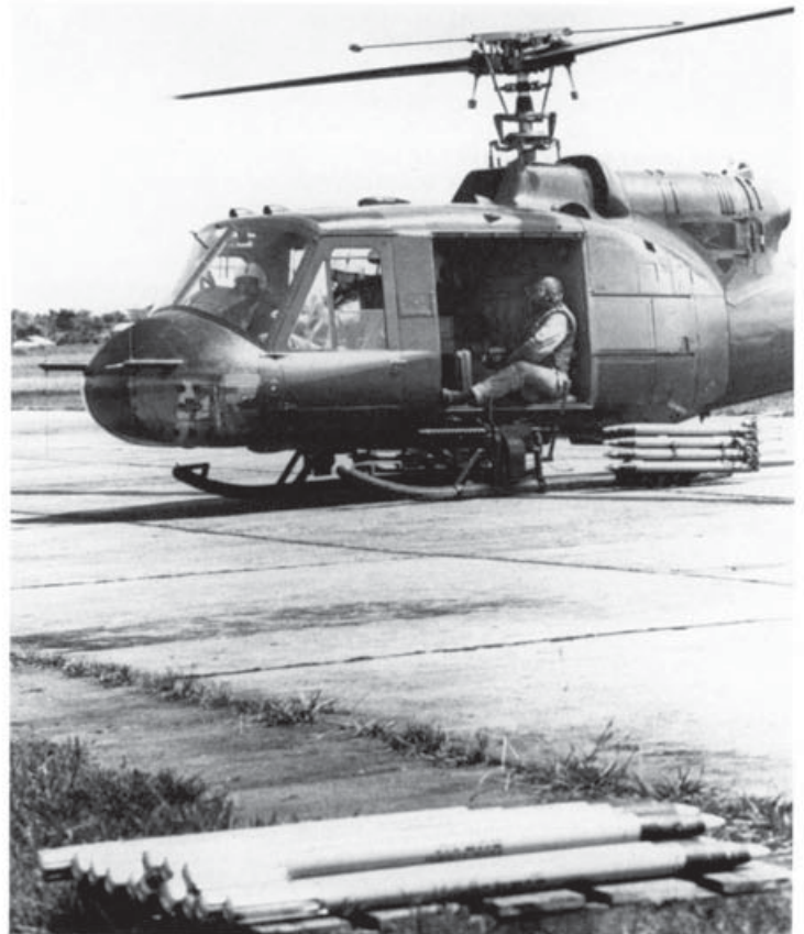
(Above) A UH-1A gunship from the provisional Utility Tactical Transport Helicopter Company (UTTCO) prepares to take off on an escort mission. The early 'A' model Hueys can be recognized by their short rotor mast and weights hanging from the blade cuffs. (Bell)
