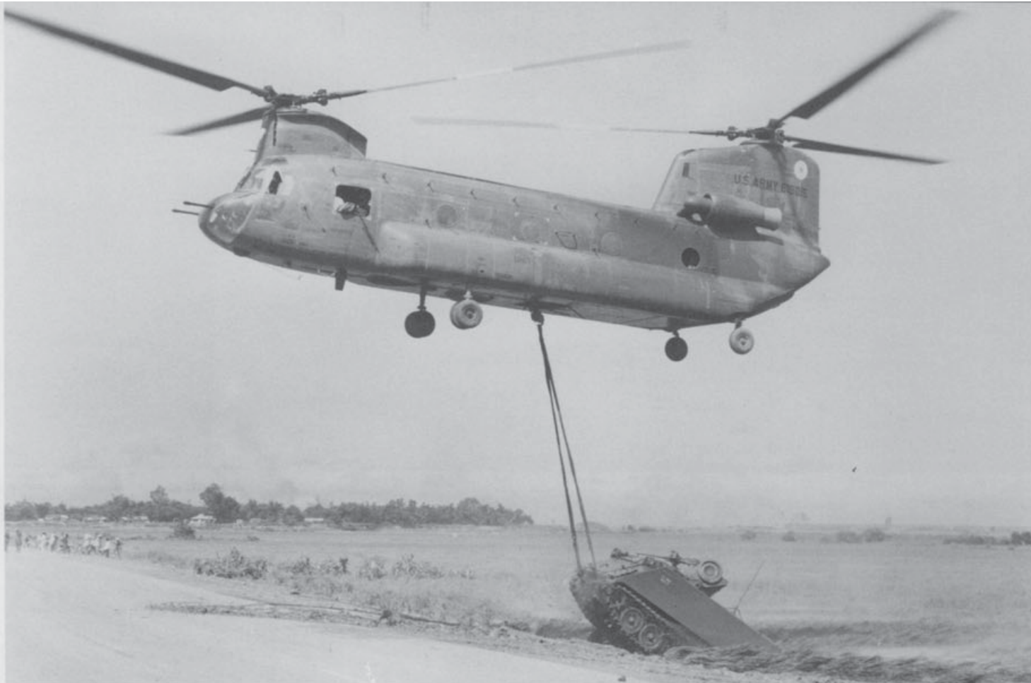
Sometimes the Army even supplied an aerial towing service. This Chinook from the 242nd MHC helps pull a mired M-113 onto solid ground near Cu Chi. Had the M-113 been completely bogged down the services of a Skycrane would probably have been required. (US Army)
