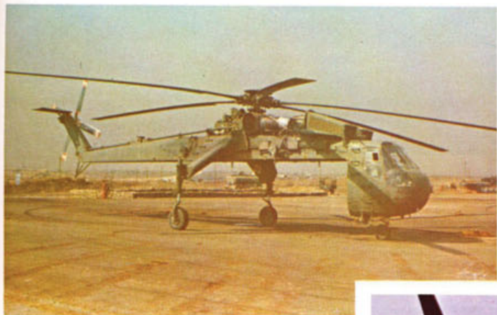
This CH-54 Skycrane from the 478th Aviation Company sits on the helopad of the 199th Infantry Brigade at Long Binh. The box shaped objects ahead of the intakes are a filter system designed to overcome the extremely dusty conditions in Vietnam during the dry season. (Mutzig)
