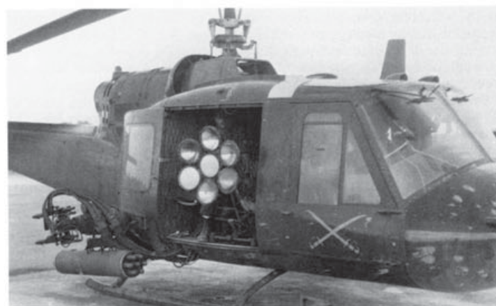
In an attempt to counter the enemy's use of darkness as a shield for infiltration, a number of Hueys were equipped with lights for night surveillance work. This UH-1B is fitted with C-130 landing lights and was used to illuminate the perimeter at Tan Son Nhut in early 1966. Helicopters so fitted were sometimes nicknamed 'lightning bugs'. (US Army)
