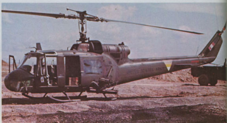
This UH-1C Gunship from 'A' Troop, 3rd Squadron, 17th Cavalry is at a forward support base. It is armed with mini-guns and 2.75 inch rockets. (Mutzig)
