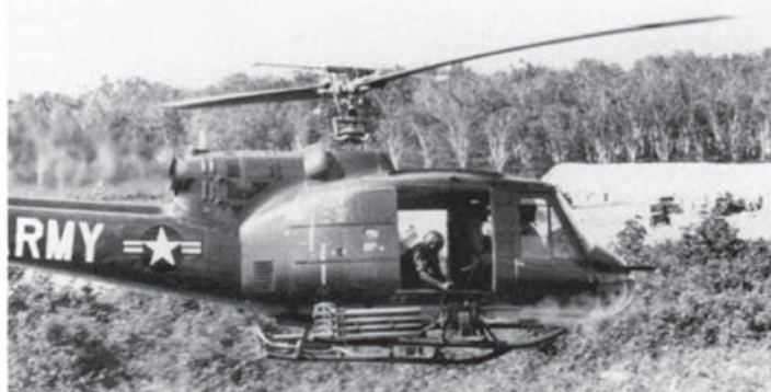
A UH-1A makes a practice run at a firing range outside of Saigon. Notice how the crew chief is holding the cocking lever. These first gunships did not have side mounts for additional machine guns as did later versions of the Huey series. (Bell)
