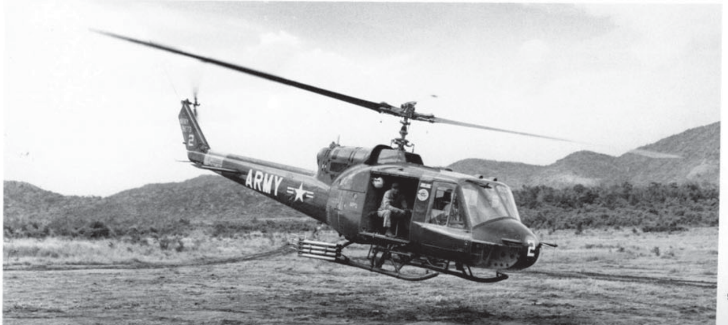
(Above) A UH-1A gunship from the provisional Utility Tactical Transport Helicopter Company (UTTCO) prepares to take off on an escort mission. The early 'A' model Hueys can be recognized by their short rotor mast and weights hanging from the blade cuffs. (Bell)
