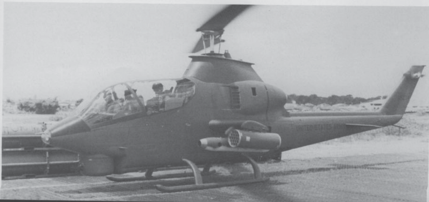
An unidentified Cobra prepares to lift off on a mission to support US troops. The mini-gun pod on the wing stub appears to have been obtained from the air force because of the camouflage paint on the lower surface. (Bell)
